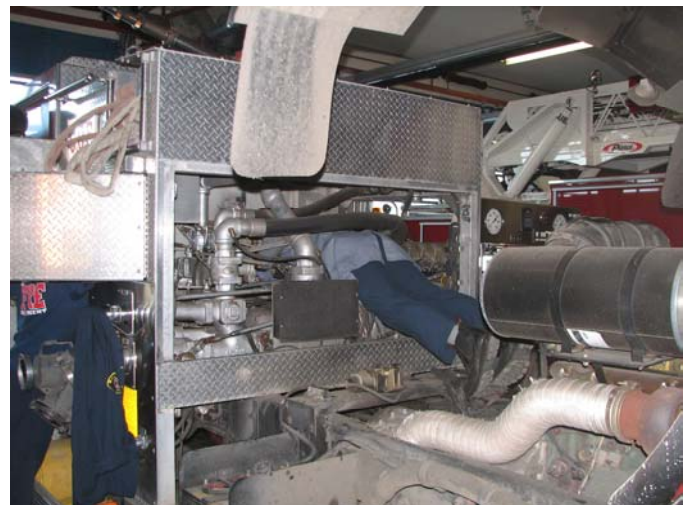
Engineer/Mechanic Skylar Thornton works to repair pump plumbing on an out of service engine.
