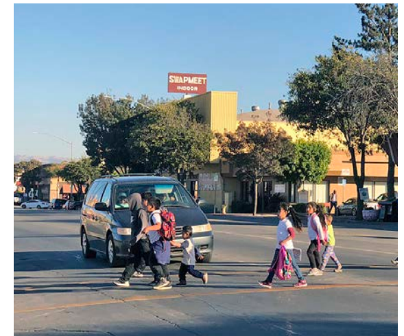
Many pedestrian crossings lack high-visibility markings.
