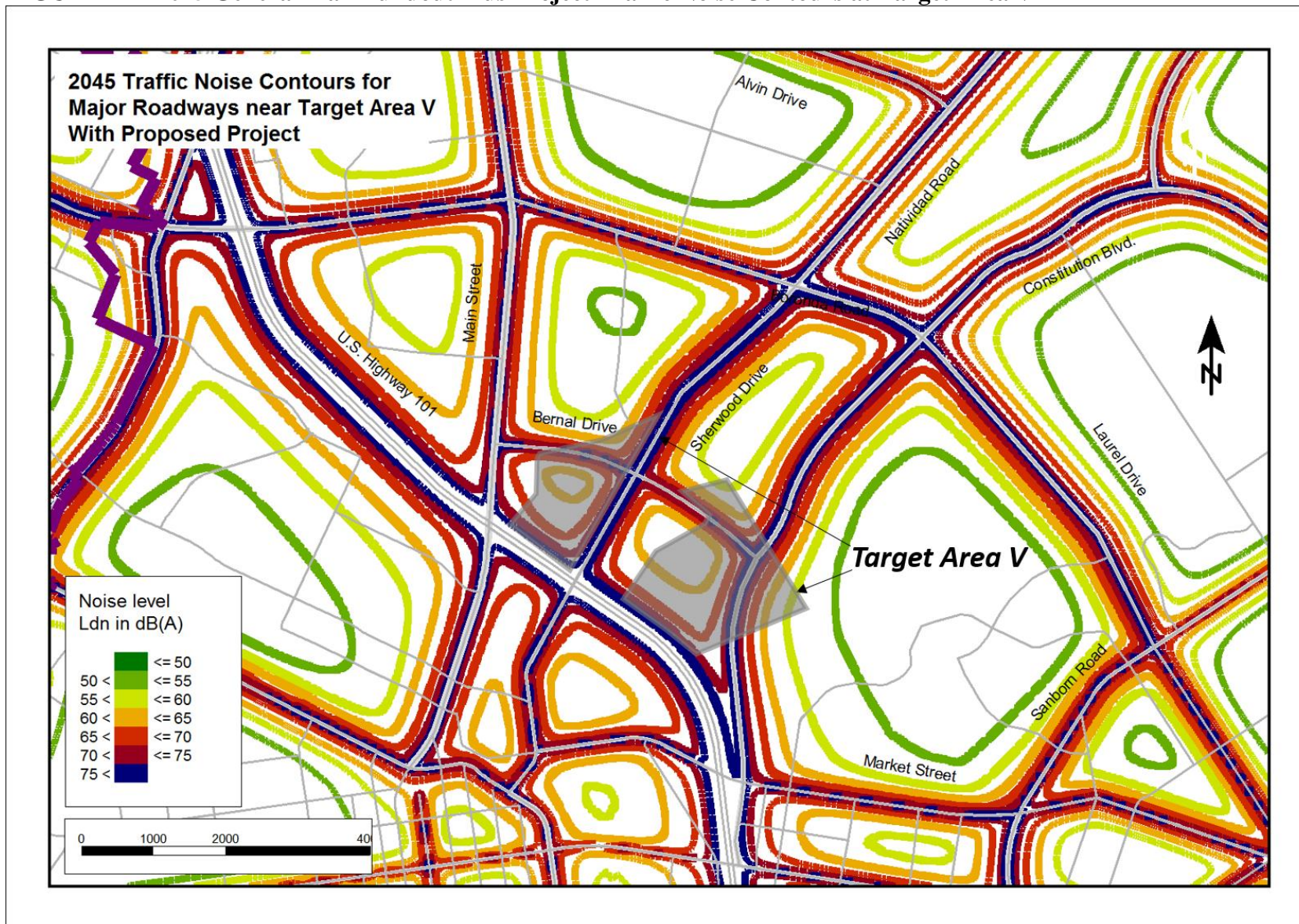
FIGURE 4 2045 General Plan Buildout Plus Project Traffic Noise Contours at Target Area V
