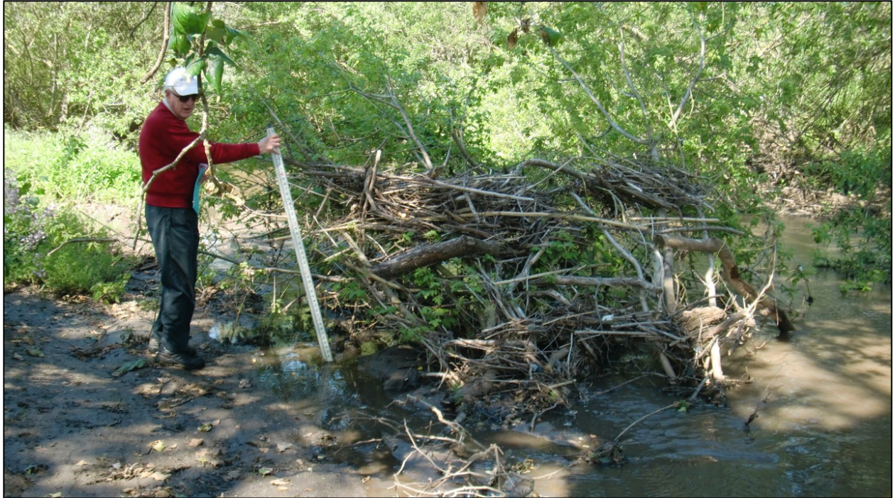
Figure 9 Streamwood and sediments transport downstream during flood conditions. Streamwood has collected on the upstream side of stream-edge riparian trees, providing an indication of how deep water was in this area. The stadia rod showed flows were about 4 feet
