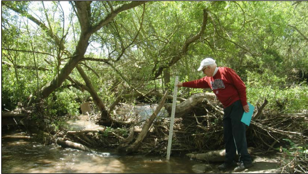
Figure 12 Streamwood deposition against roughness elements in the channel, looking downstream. High flows were ~4 feet above channel bed.
