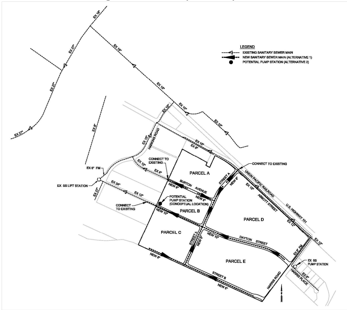
Figure 8-6: Sanitary Sewer System
