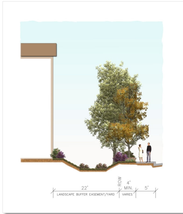
FIGURE 4-2 LANDSCAPE BUFFER EASEMENT ADJACENT TO BUILDING
