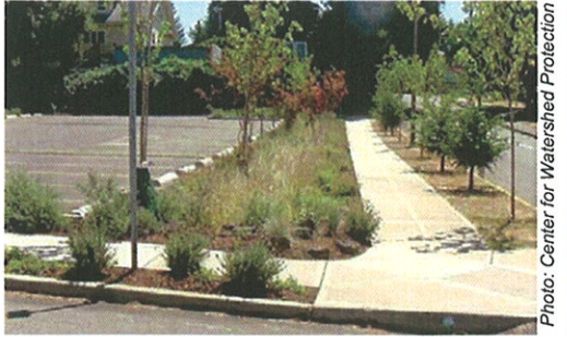
Figure 3-398: Landscape Detention Basins Located at the Edge of a Parking Lot (left photo) and in a Parking Lot Island with Turf and Shrubs and Trees (right photo)
