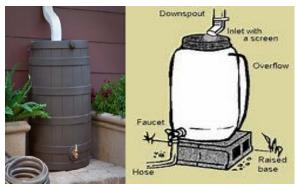
Rain Barrel Installation and Schematic Installation
