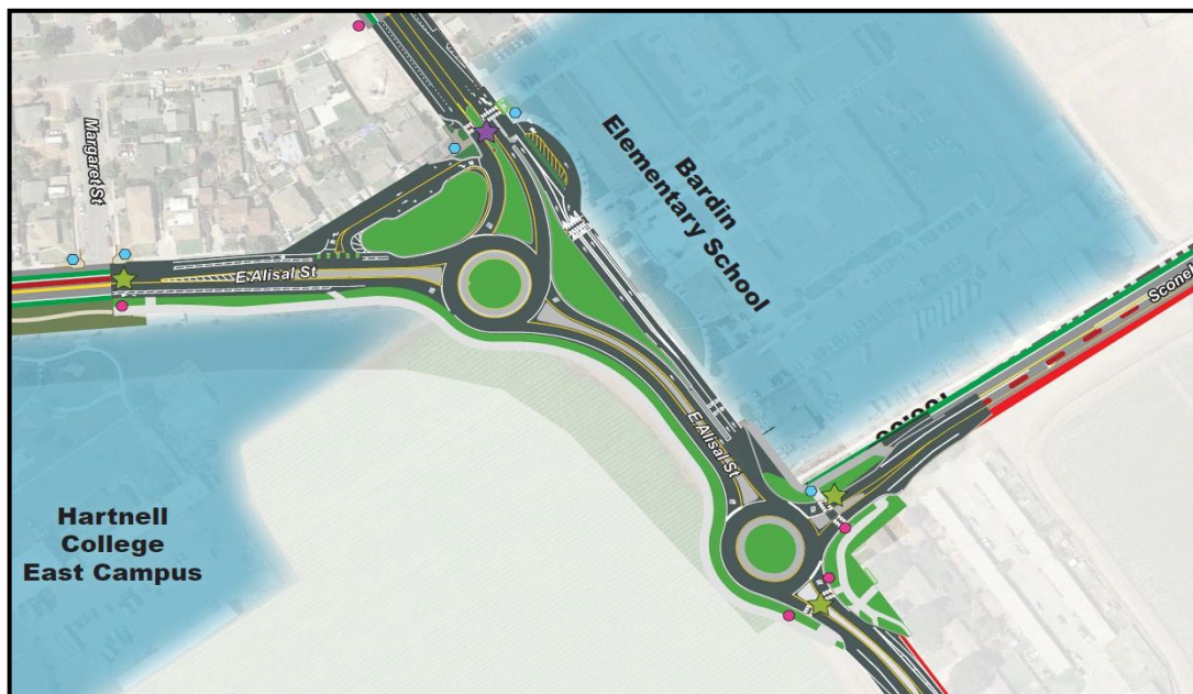
Rendering of Sch. A Improvements - Roadway Reconfiguration at Alisal St/Bardin Rd and at Sconberg Pkwy/Alisal Rd.
